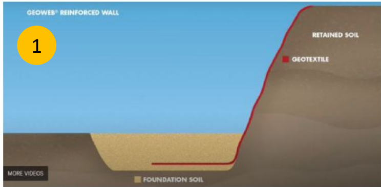
Excavate and lay terram
