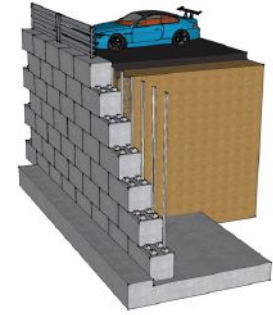
Cantilever - Reinforced Block
